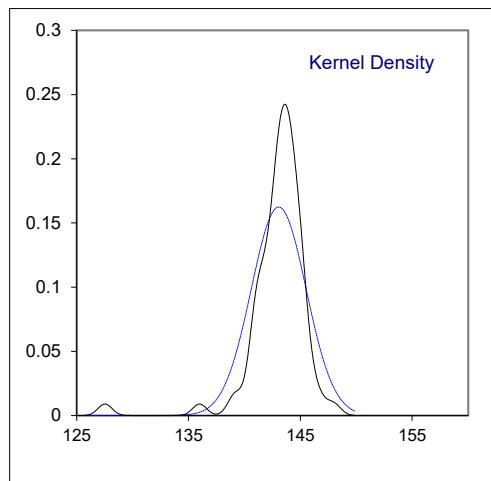
Determination of Kinematic Viscosity Stabinger at 40 °C on sample #23080; results in mm<sup>2</sup>/s
